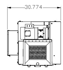
MWS-21001 NUMBER OF MOTORS: 1 DRIVE: 1 HP ELECTRIC VOLTAGE: CUTTING CHAMBER 8" X 10" CUTTERS: 5/16" WEIGHT: 450 LB SYSTEM TOTAL
